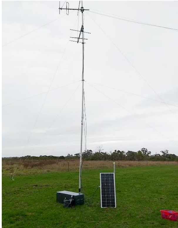
Fixed tracking station erected recently at north Western Port Bay release site, to supplement hand-held radio-tracking efforts. Photo by Ashley Herrod
